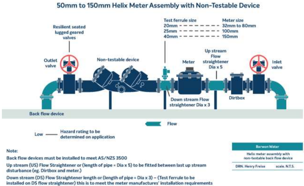
Figure 15 – 50mm to 150mm Helix Meter Assembly with Non-Testable Device
