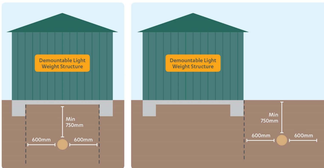
Figure 9: Shed : Demountable light weight structure
